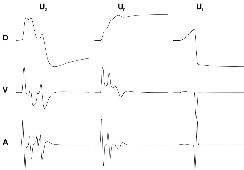
Fig. 5. Halfspace medium response to a point force in the  $x_1$  direction at a location (14.14 14.14 0.0) from a source located at (0,0, 5). In the figure  $U_z$  is in the up-direction.
