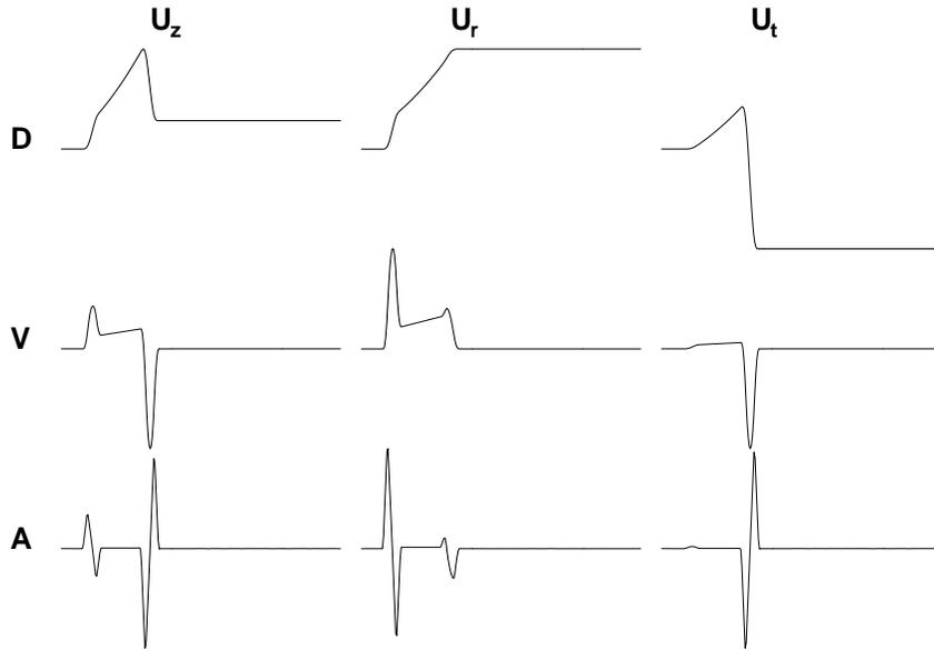
Fig. 2. Infinite medium response to a point force in the  $x_1$  direction at a location  $(14.14, 14.14, 0.0)$  from a source located at  $(0,0, 5)$ . In the figure  $U_z$  is in the up-direction,  $U_r$  and  $U_\phi$  are positive in the direction of increasing  $r$  and  $\phi$ , respectively.
