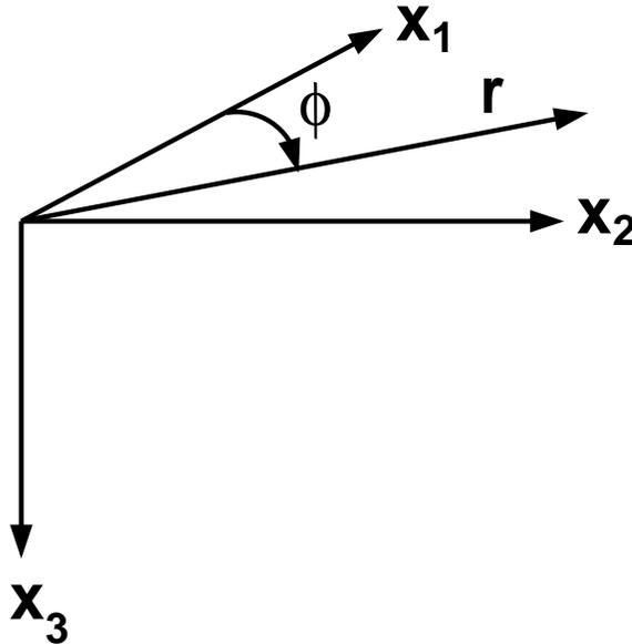
Fig. 1. Coordinate system for development of the theory. Note that the the convention for measurement at the surface of the earth is that  $z$  is positive upward. Thus the vertical component of any computed waveform will be opposite in sign to that derived theoretically for the  $z$ -positive downward coordinte system, e.g.,  $x_3$ .
