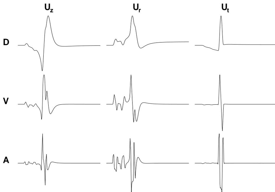
Fig. 6. Halfspace response to a moment tensor force corresponding to a shear dislocation with strike  $45^\circ$ , dip  $45^\circ$  and rake  $45^\circ$ . acting at a location (14.14, 14.14, 0.0) from a source located at (0,0, 5). In the figure  $U_z$  is in the up-direction.
