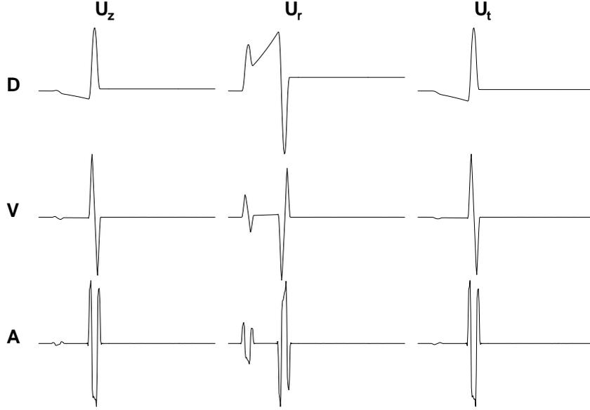
Fig. 3. Infinite medium response to a moment tensor force corresponding to a shear dislocation with strike  $45^\circ$ , dip  $45^\circ$  and rake  $45^\circ$ . acting at a location  $(14.14, 14.14, 0.0)$  from a source located at  $(0,0, 10)$ . In the figure  $U_z$  is in the up-direction.
