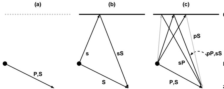
Fig. 4. Ray diagrams for wave propagation. (a) wholespace problem; (b) halfspace SH problem; (c) halfspace P-SV problem.
