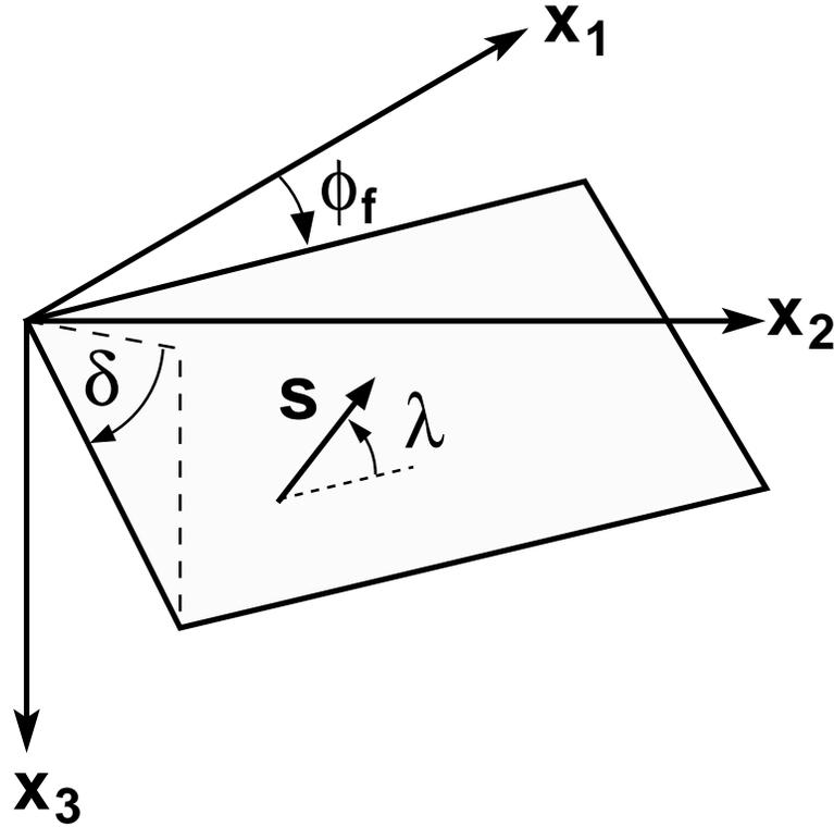
Fig. A.1. Fault plane angle convention. The  $x_1$ ,  $x_2$  and  $x_3$  axes are in the north, east and down directions.  $\phi_f$  is the strike, measured north,  $\delta$  is the dip, measured downward from a horizontal direction perpendicular to the strike, and  $\lambda$  is the rake angle indicating the direction of motion on the fault, given by the vector  $s$ . The side of the fault nearest the viewer will move in the  $s$  direction.
